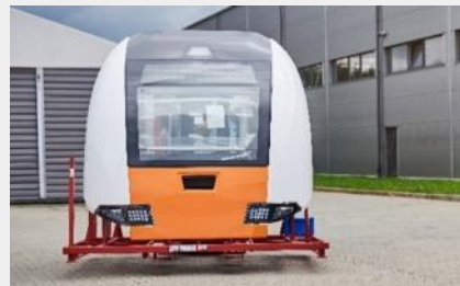
INNOCAB® Sandwich Front Cabin (incl. painting, bonding, assembly)
