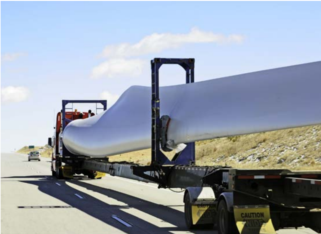
▼ Blade transport on truck, AIREX® and BALTEK® products used in wind rotor blades
