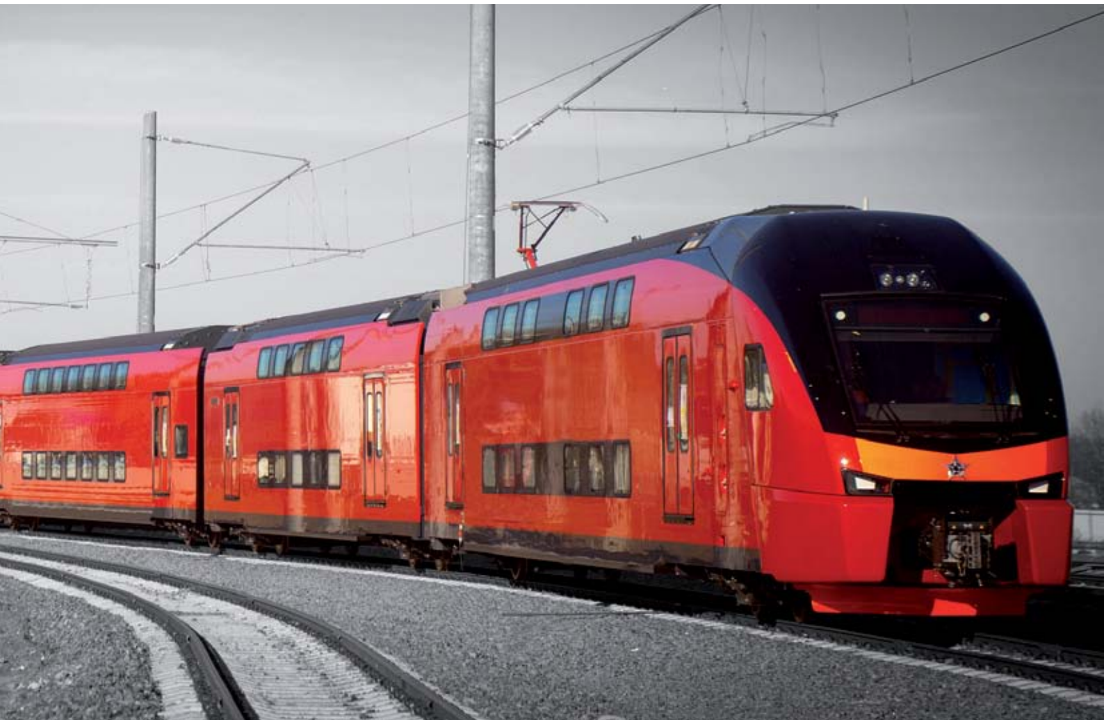
KISS double-deck electric multiple unit by Stadler Rail for the Aeroexpress, Moscow
